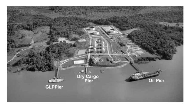
The downstream berth, next to the GLPpier, is formed by the Floating Operation Platform (POF-2) and mooring buoys, has the same configuration as the upstream berth and is 360 meters away from the oil pier.berthberth
